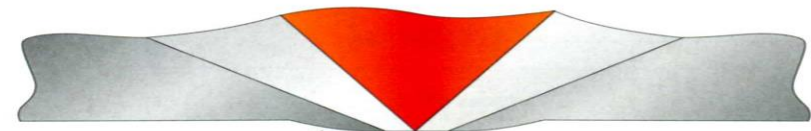
Figure 11.7 Effect of thermal expansion on gate tip heater positioning
